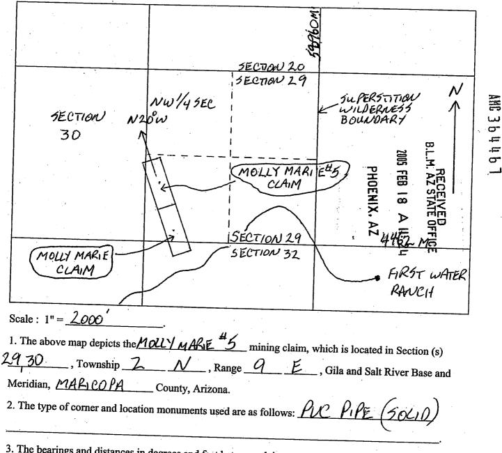
3. The bearings and distances in degrees and feet between claim corners are as depicted on the map. 4250° THE BEARING 5 AND DIFTANCES BETWEEN THE CORNERS OF THE CLAIM BEGUNNING IN THE NW CORNER OF THE CLAIM 560 FEET IN A N TO E DIRECTION TO THE NE CORNER 1460'IN A SOUTH 20°E DIRECTION TO THE SE CORNER, 560 FEET IN A STO°N TO THE SW CORNER, THEN 1460' TO THE POINT OF BEGINNING.
