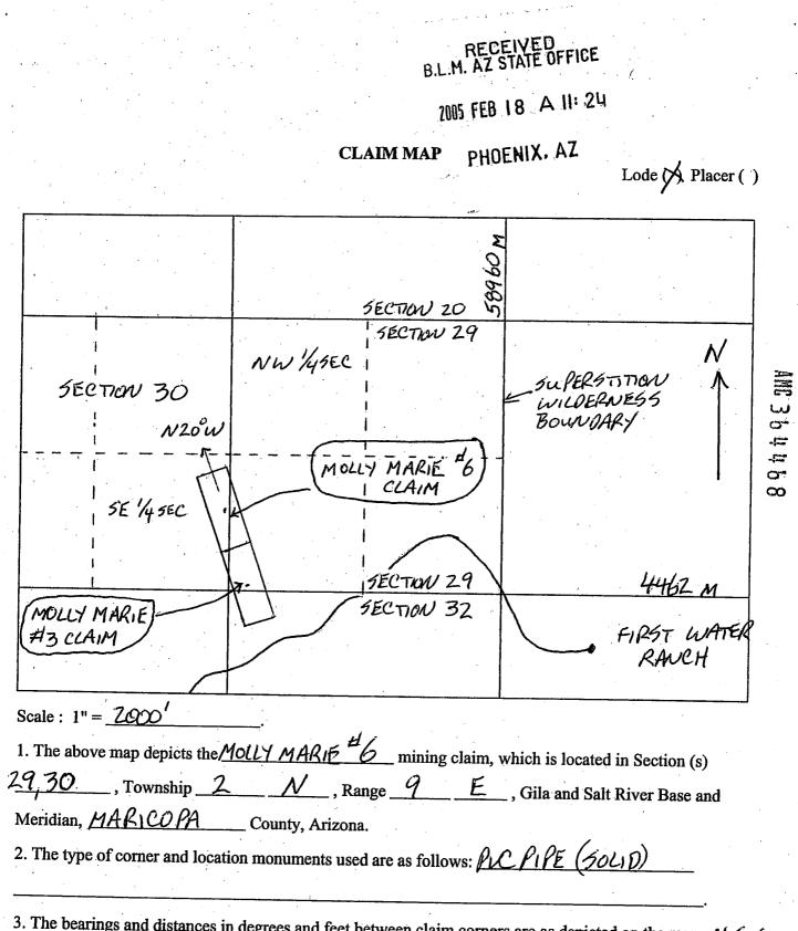
3. The bearings and distances in degrees and feet between claim corners are as depicted on the map. ALGO: THE BEARINGS AND DISTANCES BETWEEN THE CORNERS OF THE CLAIM BEGINNING IN THE NW CORNER OF THE CLAIM: 560 FEET IN A N70°E DIRECTION TO THE NE CORNER, 1460' IN A 520°E DIRECTION TO THE SE CORNER, 560 FEET IN A 570°W TO THE SW CORNER, AND THEN 1460' TO THE POINT OF BEGINNING:
